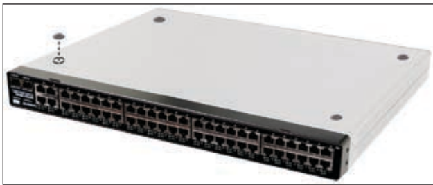
Attaching the Switch’s Rubber Feet
